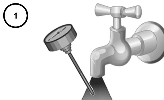
Using a thermometer, test the mixed water temperature at the nearest outlet being supplied by the valve. This should be opened to allow a minimum flow rate of 1.5 gpm (6 L/min). Allow the water to run for at least one minute to ensure the mixed water temperature has settled.
