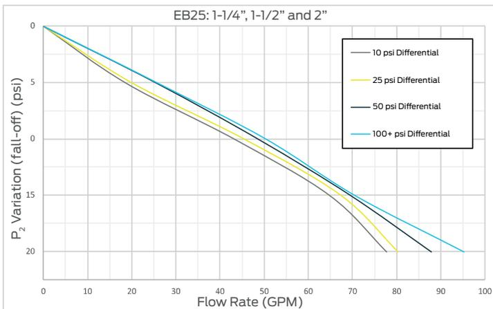
**Pressure Differential:** Difference between the inlet pressure and the PRV set pressure.
