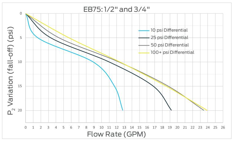
**Pressure Differential:** Difference between the inlet pressure and the PRV set pressure.
